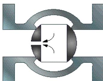
Valve with small hole drilled in ball.
