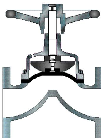
Diaphragm valve with small hole drilled in the bonnet.
