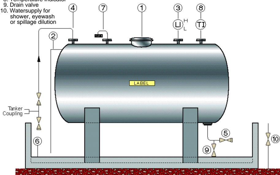
Additional features include level indicator and temperature indicator alarms. These are recommended for safety reasons. Some tanks are also fitted with a dilution connection and a mixing device. Alarm switches and thermometers must not be of the mercury type, and no oil should be used in the thermocouple well.
